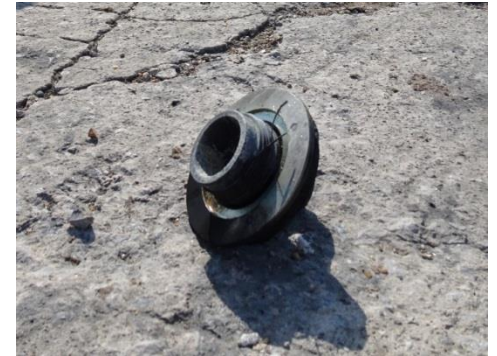
Ejected plastic plug after FCO test
