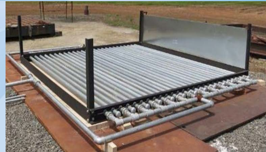
US NSWCCD 3.7 m square propane burner
