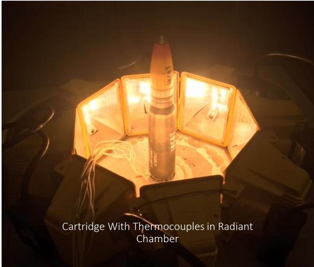
Cartridge With Thermocouples in Radiant Chamber
