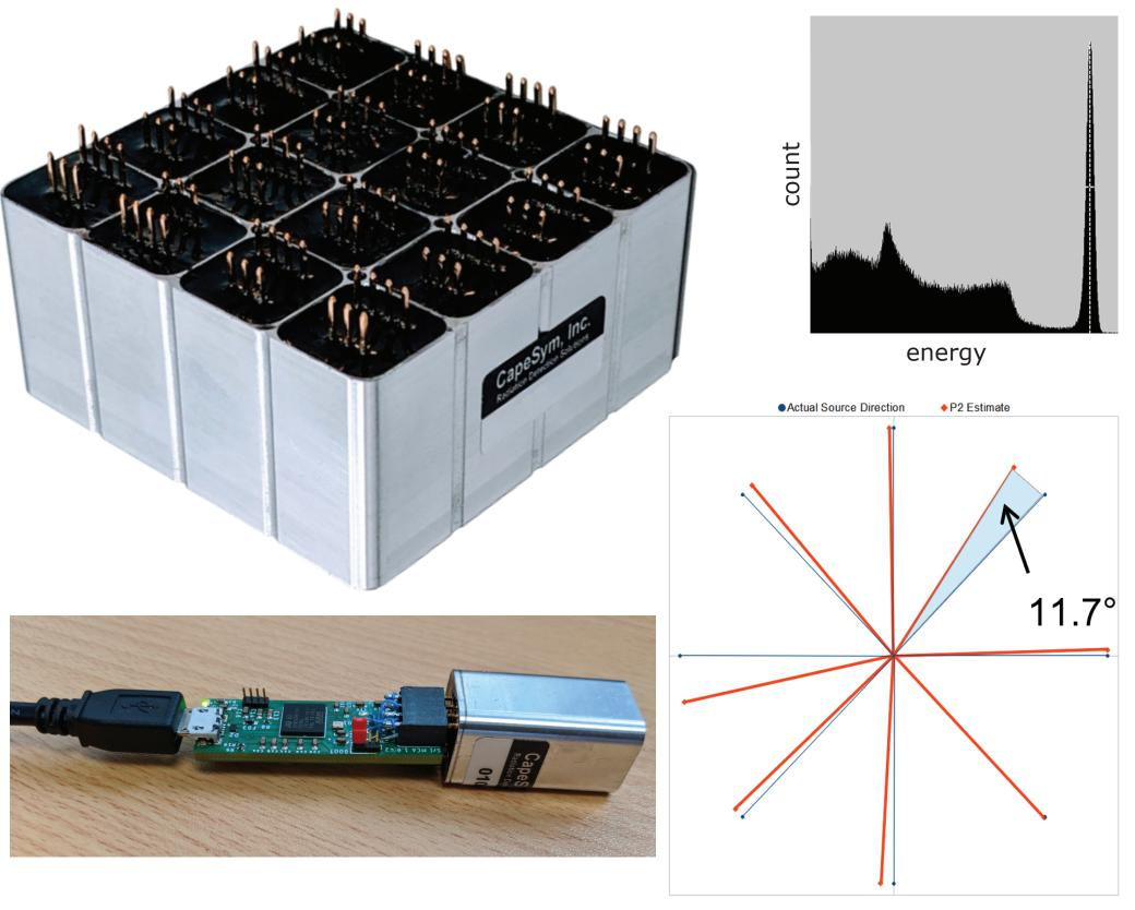
**Custom directional 16 module radiation** sensor increases detection sensitivity and enables rapid source localization
