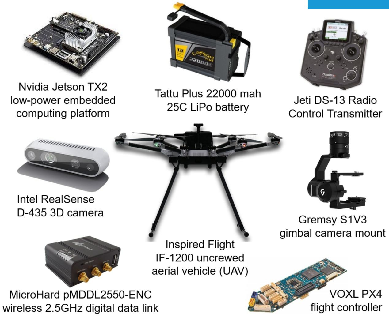
Integrated off the shelf components enable low cost, reliable autonomous capabilities
