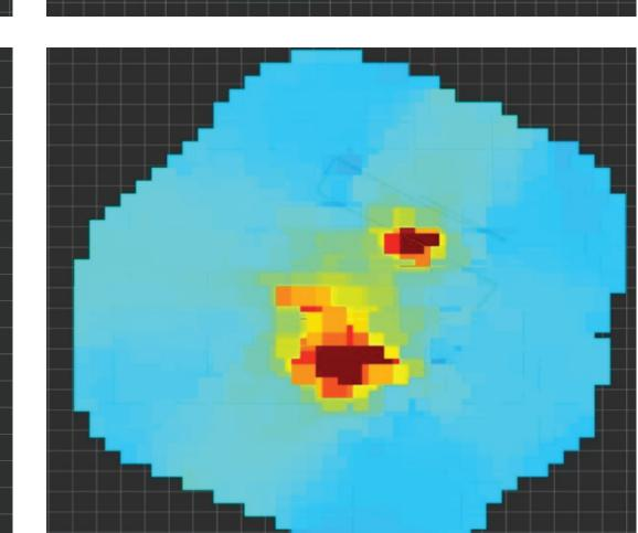
Radiation heatmaps generated in real time using a spiral search for one source (top) and a raster pattern for two sources (bottom)
