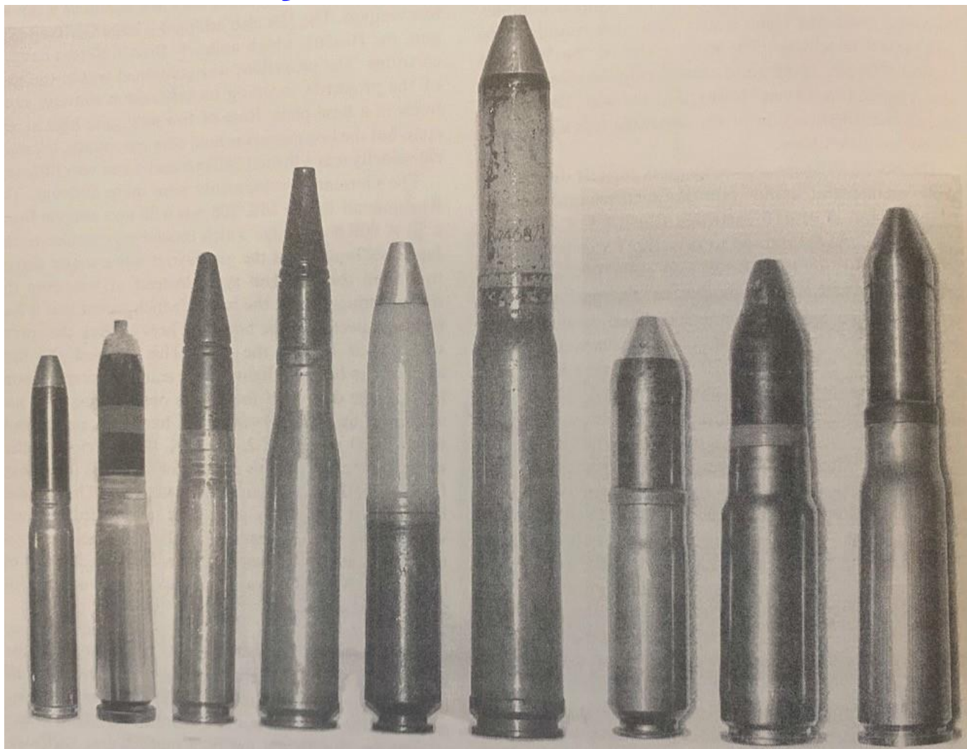
20 – 30mm Cannon Cartridges: 20 x 110 Hispano, 23 x 106 Madsen, 23 x 115 VYa-23, 30x90 Mk 108, 30x184 Mk 103, 30x114 IJA Ho0155, 30x122 IJN Type 5
