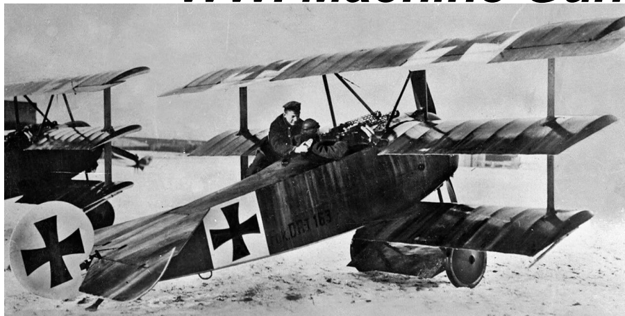
Fokker Dr.I MG08/15 8mm machine guns
