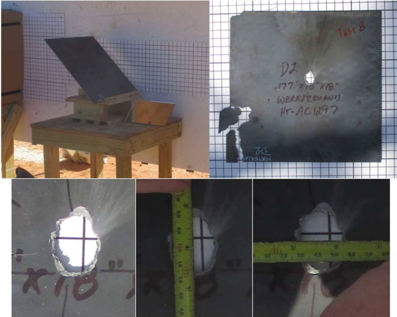
Fig. D8. RT21-478: D2 Tool Steel RC60 0.177" Thick, 45 Degrees Obliquity
