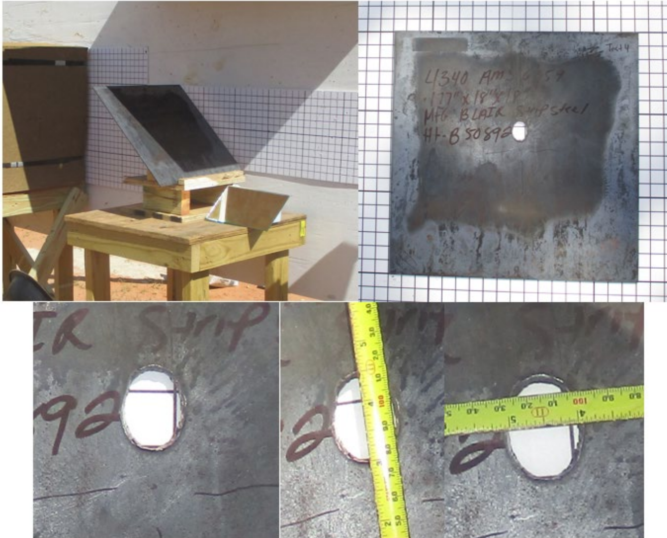
Fig. D4. RT21-472: 4340 RC38 Steel 0.177" Thick, 45 Degrees Obliquity
