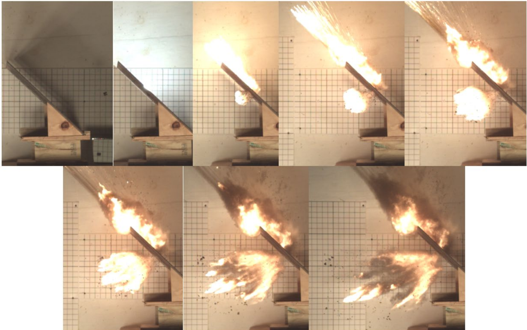
Fig. C4. RT21-472 (0.177", 4340 RC38, 45° Obliquity) high speed video frames at -120us, 0us, 40us, 80us, 120us, 160us, 240us, 320us
