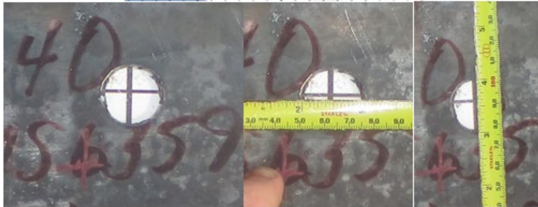
Fig. D1. RT21-469: 4340 RC38 Steel 0.125" Thick, 0 Degrees Obliquity
