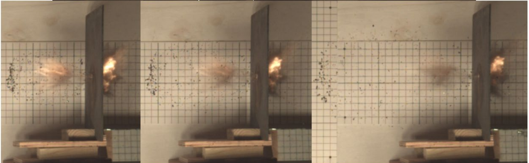
Fig. C2. RT21-470 (0.250", 4340 RC38, 0° Obliquity) high speed video frames at -100us, -50us, 0us, 50us, 100us, 150us, 200us, 300us
