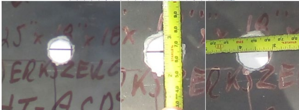
Fig. D5. RT21-473: D2 Tool Steel RC60 0.125" Thick, 0 Degrees Obliquity
