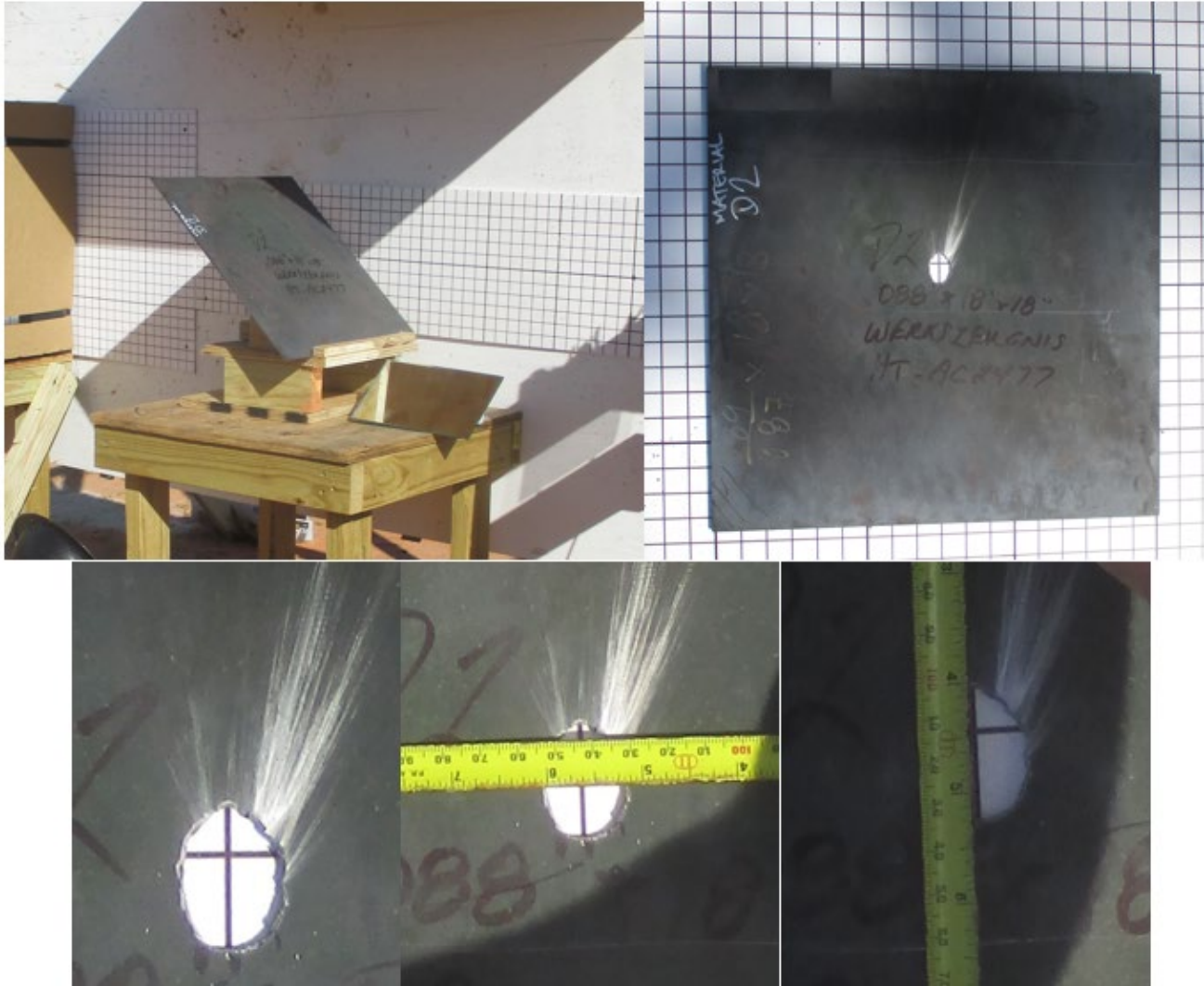
Fig. D7. RT21-475: D2 Tool Steel RC60 0.088" Thick, 45 Degrees Obliquity
