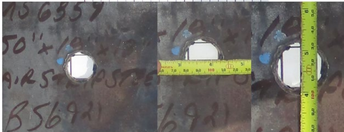
Fig. D2. RT21-470: 4340 RC38 Steel 0.25" Thick, 0 Degrees Obliquity
