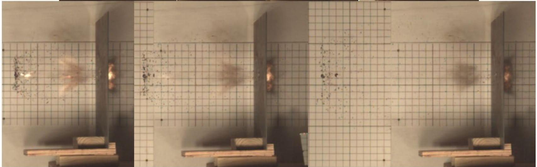
Fig. C1. RT21-469 (0.125", 4340 RC38, 0° Obliquity) high speed video frames at -100us, 0us, 50us, 100us, 150us, 200us, 300us
