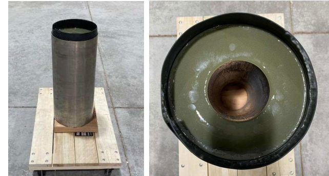
Aluminized HTPB Surrogate Rocket Motor Fabricated by R3 Aerospace
