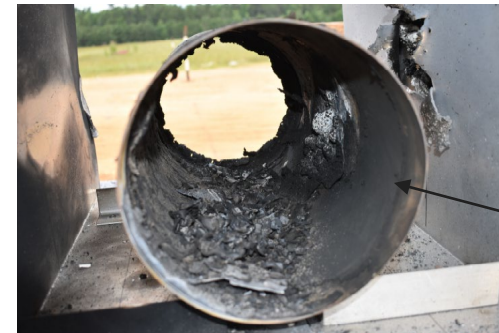
(U) Burnt out motor case still intact
