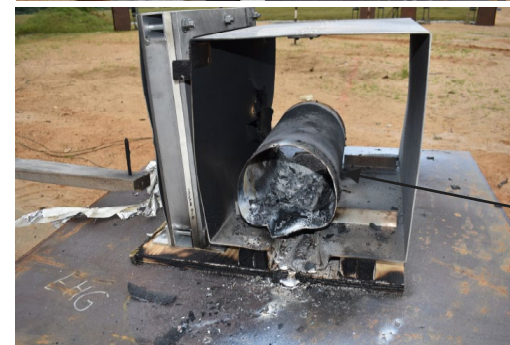
Burnt out motor case still intact
