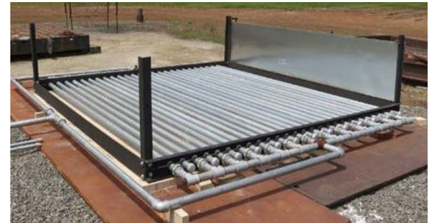
US NSWCCD 3.7 m square propane burner
