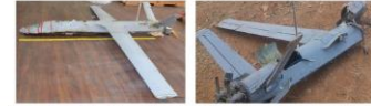
Figure 1. Reconstruction of Samad-2, length of 2.80 m (left); Samad-1 including details of the airfoil shape at the wing root (right). 15
