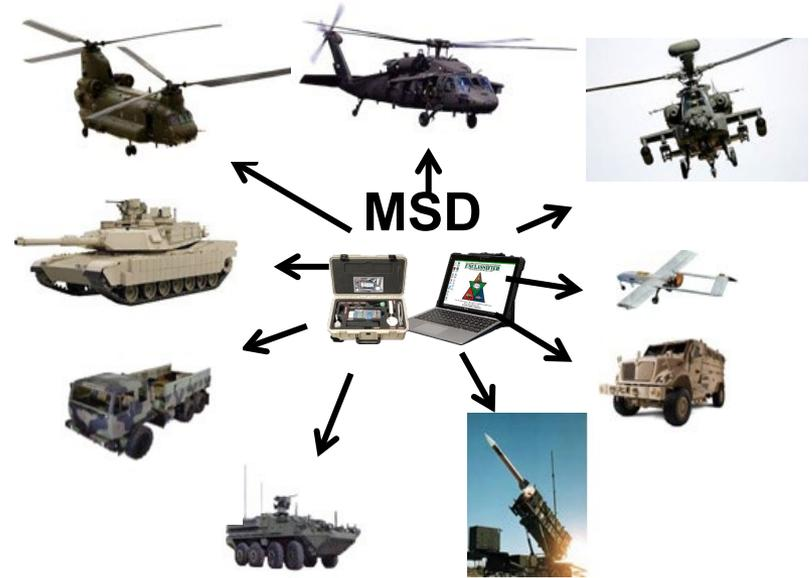
Performs quick diagnoses and fault isolation on the Army's fleet of Electronic, Tactical Wheeled, Armored Fighting, and Aviation weapon systems
