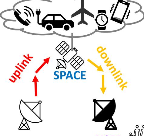
The ground segment is comprised of ground-based elements of a space system used by operators and support personnel, as opposed to the space segment and user segment.
