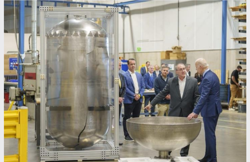
Lockheed COO, Frank St. John shows President Biden large components produced via Directed Energy Deposition, a near-net shape AM technology. This process is promising for replacing forging for critical launch components including cryogenic storage tanks. However, few companies are qualified to build parts by DED.
