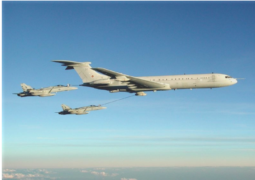
Pictured: U.S. F/A-18 Hornets received fuel from British VC-10 tanker due in part to STANAG 3447, "Aerial Refueling Equipment"
