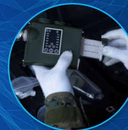
JCAD Joint Chemical Agent Detector
