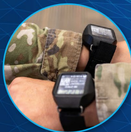
JPD-I Joint Personal Dosimeter – Individual
