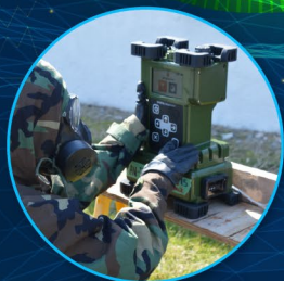
AVCAD Aerosol and Vapor Chemical Agent Detector
