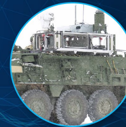
VIPER Vehicle Integrated Platform Enhanced Radiation Detection, Indication and Computation
