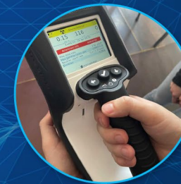
RIID Radio Isotope Identification Detector
