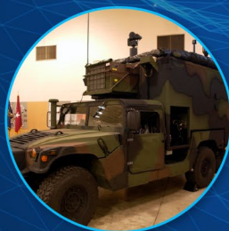
JBPDS Joint Biological Point Detection System
