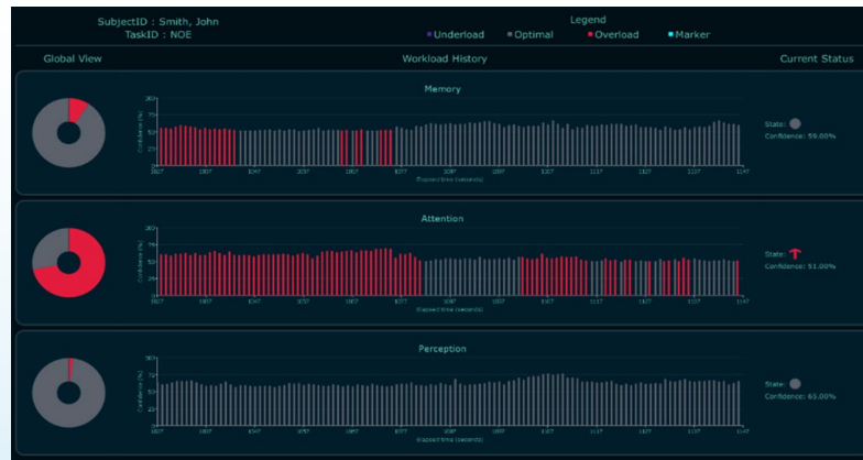
Real-time dashboard for representing cognitive load predictions for 1 st gen NGC classifiers. Red is overload, gray is adequate load, and the height of each bar is the confidence in the estimate.
