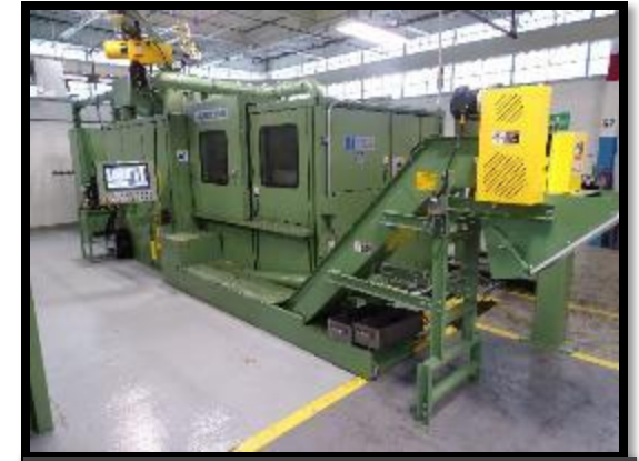
Component Cold Heading
